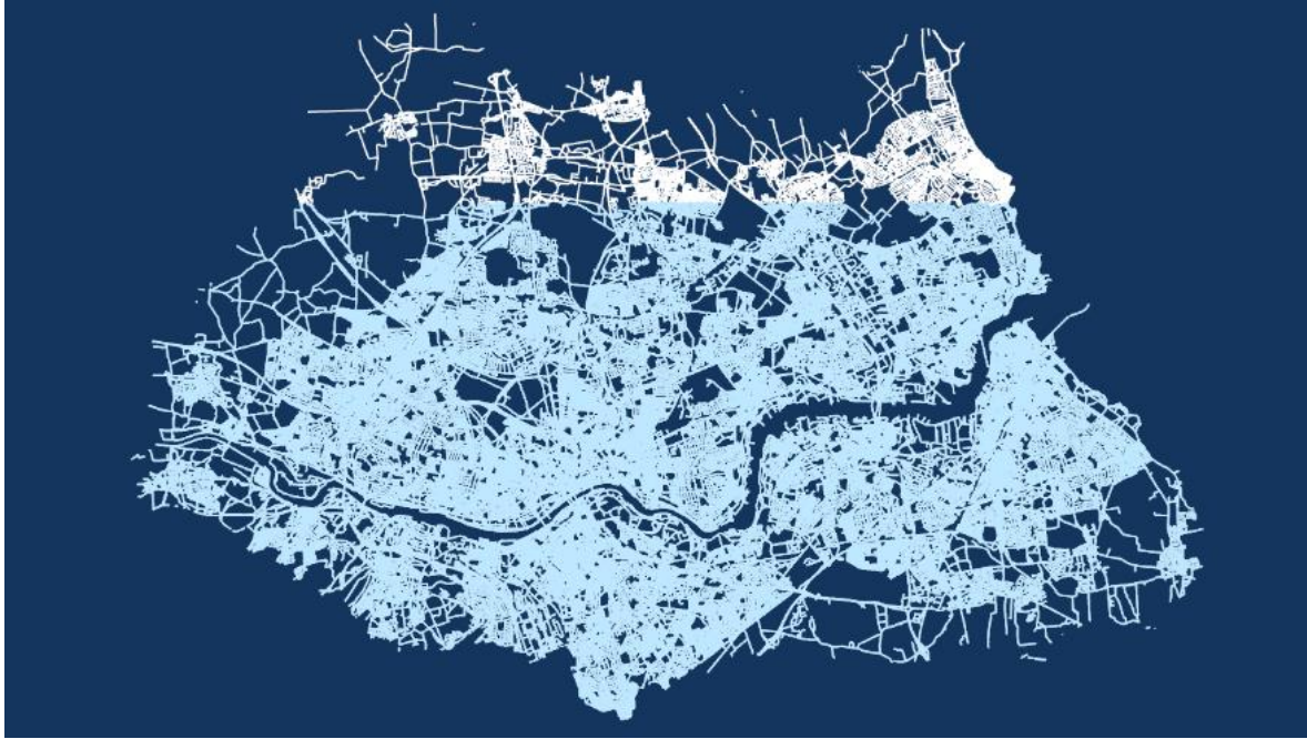
Figure 5 Shapefile size limit for the Edges dataset (white region was cut during export to shapefile in ArcGIS)
